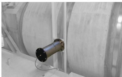
NHK for loosening adhesions on rotary kiln
