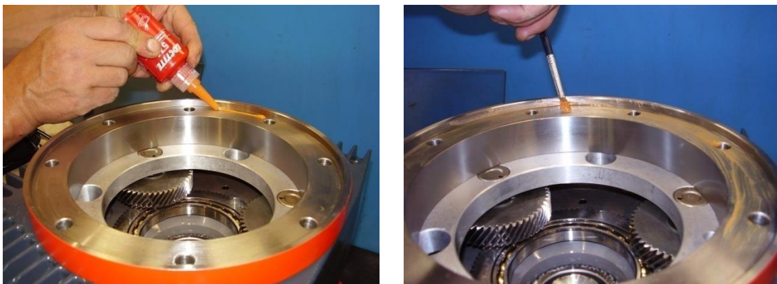
Sealing of the intermediate flange before mounting the motor flange.
